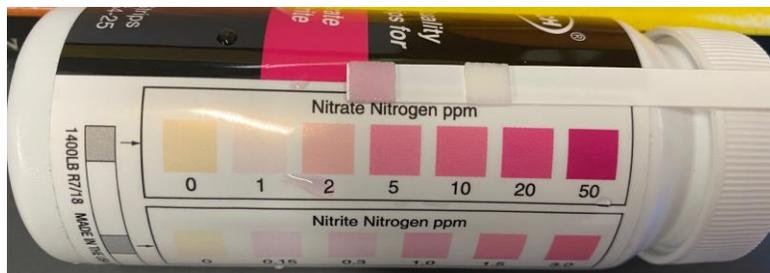
This summer I plan to visit some farms and use this test kit to rapidly estimate nitrate-N and nitrite-N ranges in the irrigation water. I also plan to send those water samples to our water analysis lab to know the exact numbers, which can be used to compare with the estimated ranges. It is recommended that our growers can try those strips for knowing their groundwater nitrate-N range in a fast way.
